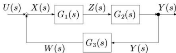
$$\begin{aligned} X(s) &= U(s) - W(s) & Z(s) &= G_1(s)X(s) \\ Y(s) &= G_2(s)Z(s) & W(s) &= G_3(s)Y(s) \end{aligned}$$
